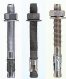
ICCONS® THRU-BOLT<sup>™</sup> PRO is a pre-assembled torque controlled mechanical stud anchor, which when tightened draws the tapered end of the bolt into the expander clip expanding it to create expansion forces against the wall of the hole.
